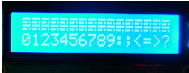
Figure 2: LCD Display: The first row displays ASCII 0 to 19, the second row displays ASCII 48 to 67
