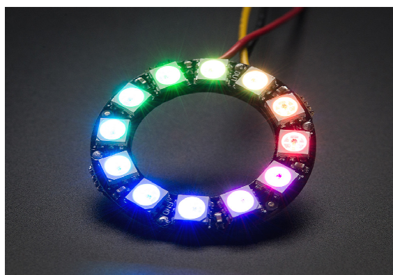
Figure 6: What the NeoPixel looks like when outputting a rainbow
