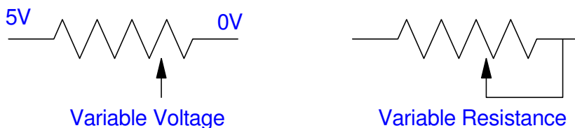
Two common configurations for potentiometers
