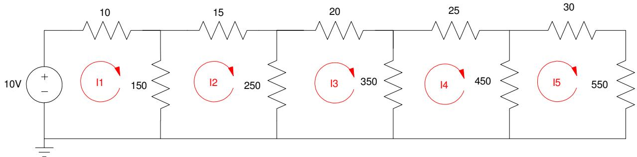
Use conservation of voltage: the sum of the voltages around any closed loop is zero
