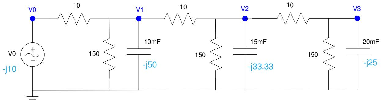
b) Write the voltage node equations
