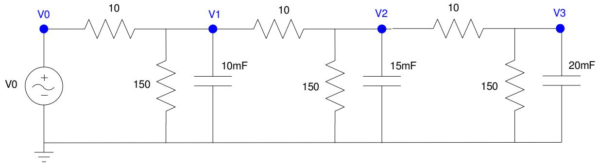
a) Determine the impedances of each element at 2 rad/sec
