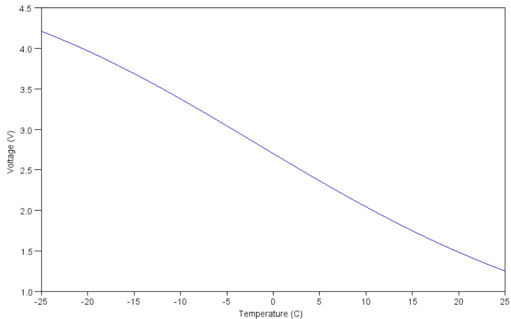
3) Over the range of -25C to +25C, determine a linear calibration curve fit as
