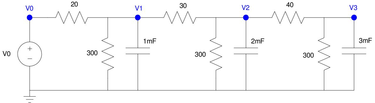
a) Determine the impedances of each element at 0 rad/sec
